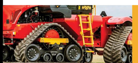
A right hand ladder gives you access to the engine air cleaner for quick servicing. The ladder also helps with right side fueling and provides access to the egress door and folds up and out of the way when not in use.
